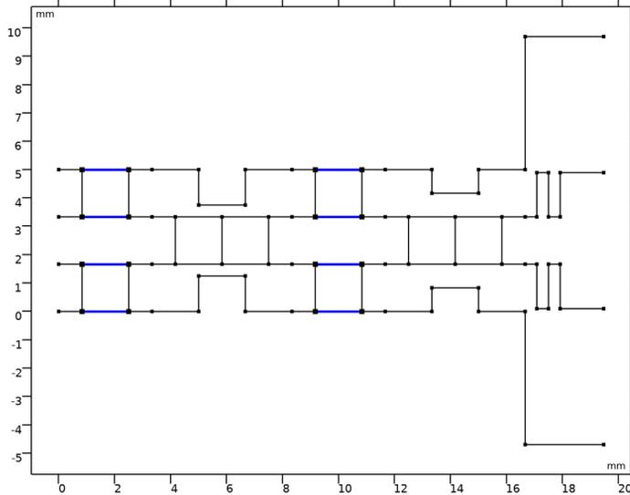
Set the impedance of the selected transmission lines (branch-lines in the 90 degree hybrid) to  $Z_0/\sqrt{2}$  by adjusting the distributed inductance and capacitance values.
