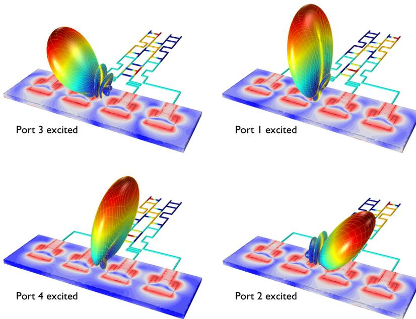
Figure 11: The far-field radiation pattern of a  $4 \times 1$  microstrip patch antenna array connected to the butler matrix beamforming network. The antenna model is not included in this example.
