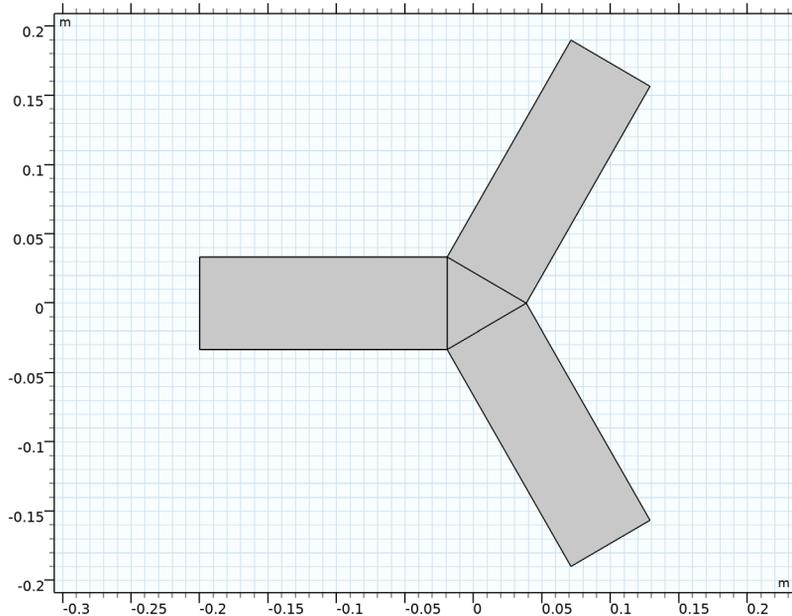
Rotate the newly created triangle 180 degrees and use one scaled copy of it to create linear fillets for impedance matching. Use another scaled copy to define the ferrite.
