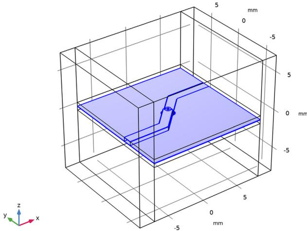
**Perfect Electric Conductor** includes all metallic surfaces: microstrip line, metalized via, via-pad, and ground plane. Make sure that the anti-via pad on the ground plane is excluded.
