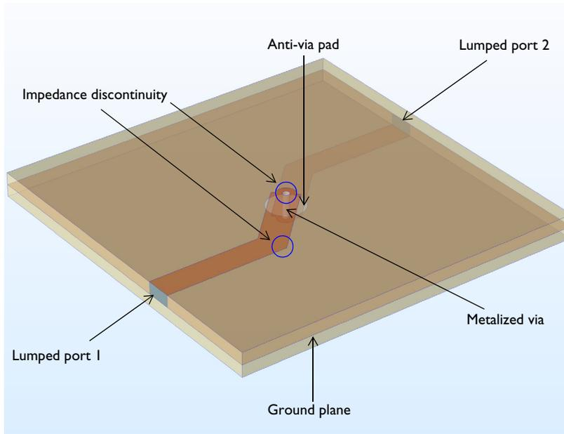
*Figure 1: A microstrip line on a multilayer circuit board. A 20 mil (0.508 mm) microwave substrate is used for each dielectric layer. The ground plane with an anti-via pad is located between two dielectric layers. The top and bottom microstrip lines are connected with a metalized via hole.*
