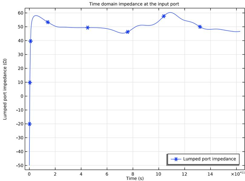
The impedance at lumped port 1 fluctuates around 50 Ω.
