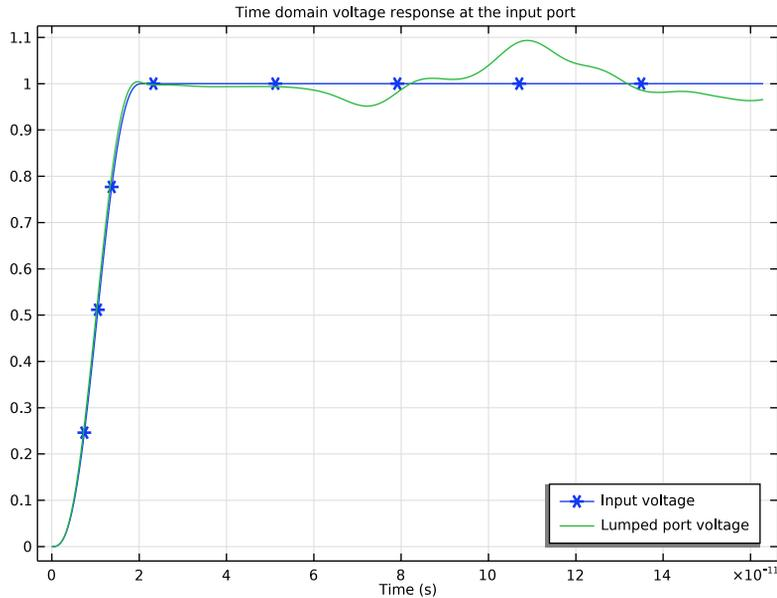
The plot shows the input and measured voltage at lumped port 1. The fluctuation in the measured voltage at lumped port 1 indicates that the reflected wave from the discontinuities causes the signal distortion. The discontinuities are at the bent microstrip line and metalized via hole.
