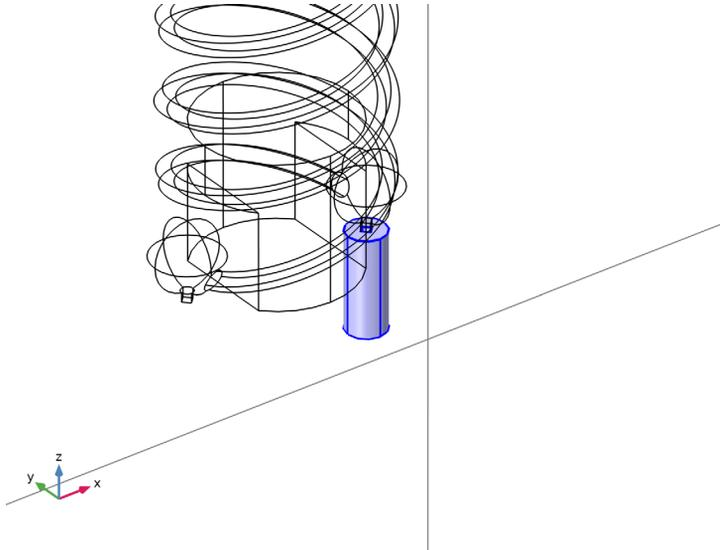
Add a selection for the model analysis domain, which is the complement of the Metal selection. So, the inside of the metal structure is not part of the model space.
