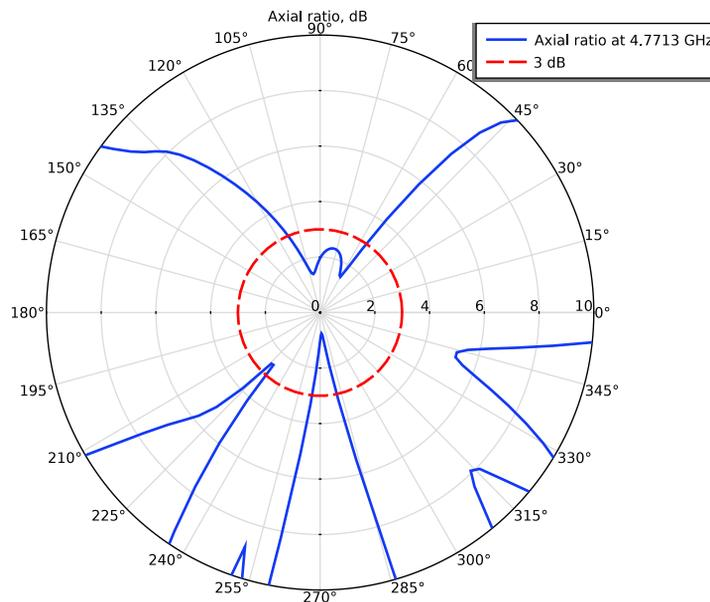
the axial ratio plot shows how much the antenna is circularly polarized. When it is characterized as the perfect circular polarization, the axial ratio is 1 or 0 dB. When it is below 3 dB (inside the red circle), it is typically regarded as a circular polarization. In
