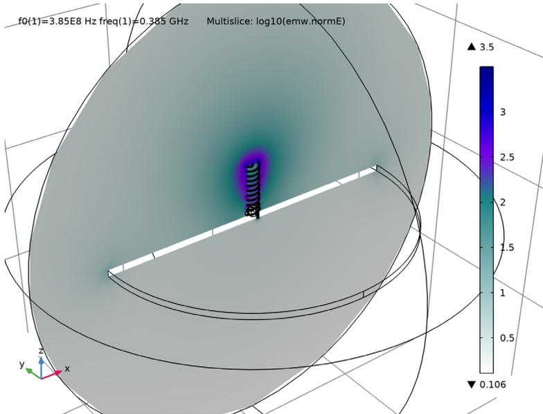
Figure 3: Log-scaled electric field magnitude around the antenna at 385 MHz.
