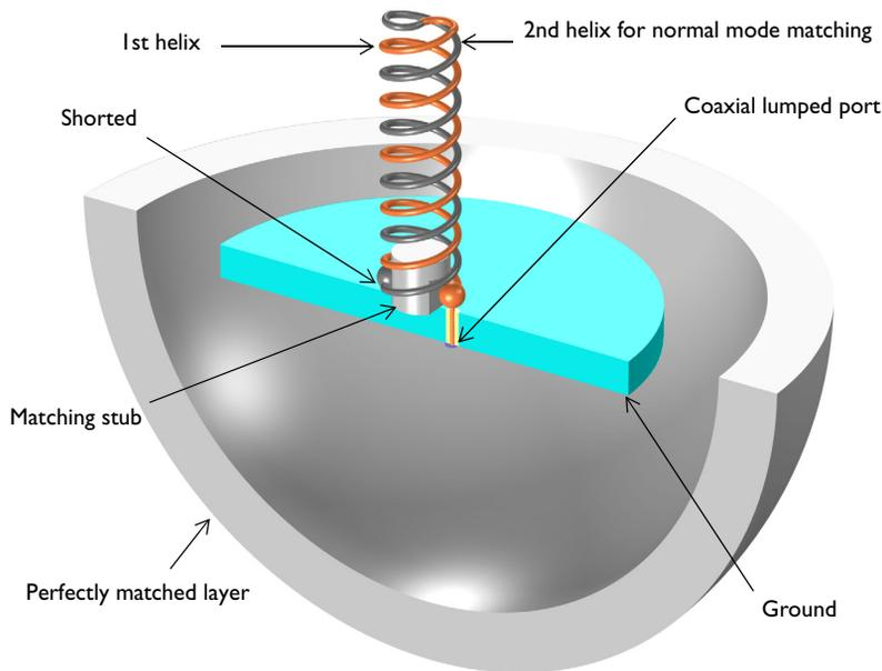
*Figure 1: Each end of the two-arm helix is connected to a coaxial cable feed and ground plate. A region of free space bounded by a perfectly matched layer (PML) surrounding the antenna. The ground plate and PML are partially visualized.*
