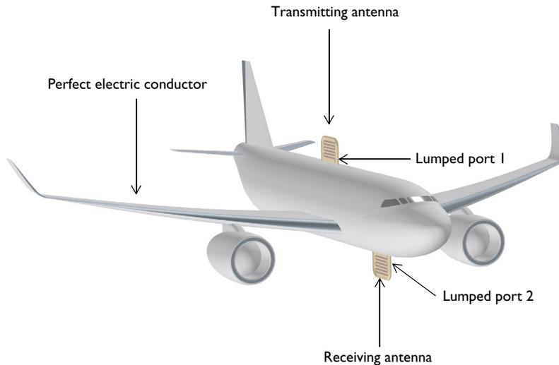
*Figure 1: An airplane with ~20 m length of fuselage is simply depicted as an all-metallic structure except for the antenna enclosure. The surrounding air domain and perfectly matched layers are not shown.*
