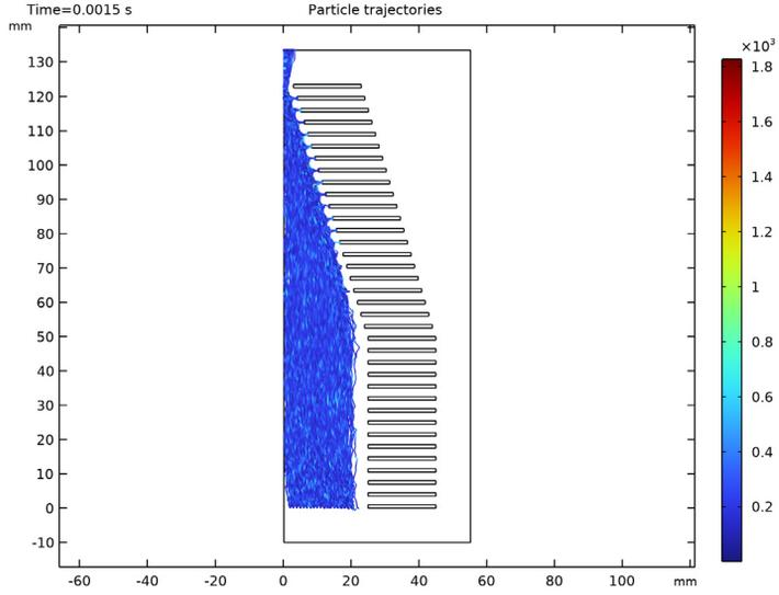
Figure 2: The trajectories of positive ions in the funnel.
