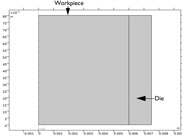
Figure 1: Geometry of the workpiece (pharmaceutical powder) and die.
