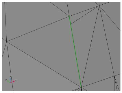
On one side of the slit (on the left side of the green edge in the figure), there is one triangle element, whereas on the other side there are two elements. Since the import functionality cannot partition elements or add new ones, the mesh edges on the two sides of the slit could not be merged even with the larger tolerance.
