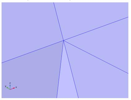
The mesh vertices are now merged, thereby eliminating the hole and the edge adjacent to it. You can easily verify this by inspecting the number of edges listed in the **Information** node or by turning off the mesh rendering temporarily.
