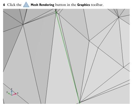
The selected edge is next to a very narrow slit that has the same number of edge elements on both sides. Zoom in further on the upper center of the image above, a bit
