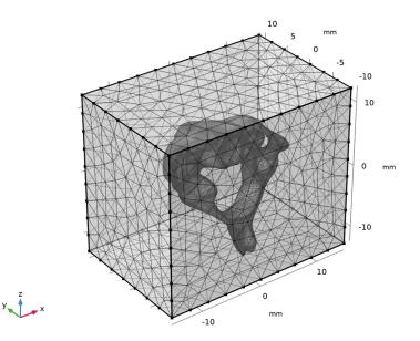
3 Rotate the mesh in the Graphics window to check that the vertebra is fully contained in the block, the two meshes should not intersect. Click the Go to Default view button. You can also use mesh Statistics to check that only triangle elements were imported for the block.
