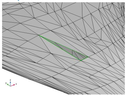
The original triangular hole remains since it is larger than the automatically determined tolerance for **Fill Holes**. Measure the perimeter of the remaining hole to obtain an estimate for the tolerance value to use with the **Fill Holes** feature. The edge should already be selected, but select it again if needed.
