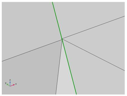
The corners of the triangular elements do not match since the corresponding mesh vertices were not merged during the import. To fix this, reimport the file using a larger tolerance.
