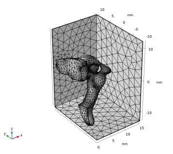
When generating a new mesh with the **Free Triangular** operation, smooth surfaces are first created in the background, based on the original mesh. These surfaces are then used when the new mesh is generated. See the discussion in the section *Comparing the Meshed Geometry with the STL Mesh* in the tutorial *STL Import 1* — *Generating a Geometry from an Imported Mesh* for more information on how the **Relative** simplification tolerance influences the shape of the faces to remesh.
