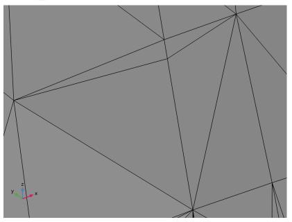
The slit has been repaired by introducing a mesh edge on the left side of the slit, merging the two sides of the hole, and removing the edge.
