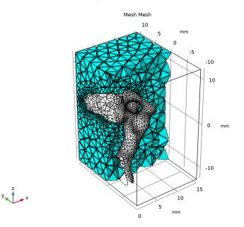
Set the **Element scale factor** to a value smaller than 1 to inspect how individual mesh elements are connected, as you can then see the parts of the surrounding elements that would otherwise be hidden behind the first layer of elements in the view. You can enter a value larger than 1 to increase the size of the elements in the plot. Use this when you need to inspect the shape of individual elements that are really small.
