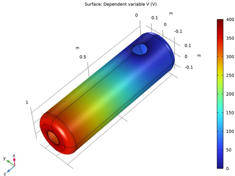
Figure 1: Electric potential distribution across the surface (V).
