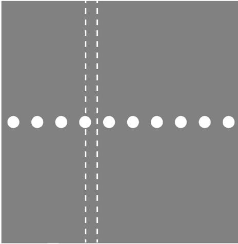
*Figure 2: Using symmetry to reduce computation time and complexity. The model describes one section of the array of heating tubes (indicated by the dashed lines).*
