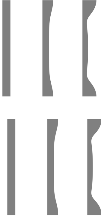
Figure 3: Comparison of solutions obtained using level-set (top row) and the moving mesh (bottom row) methods.
