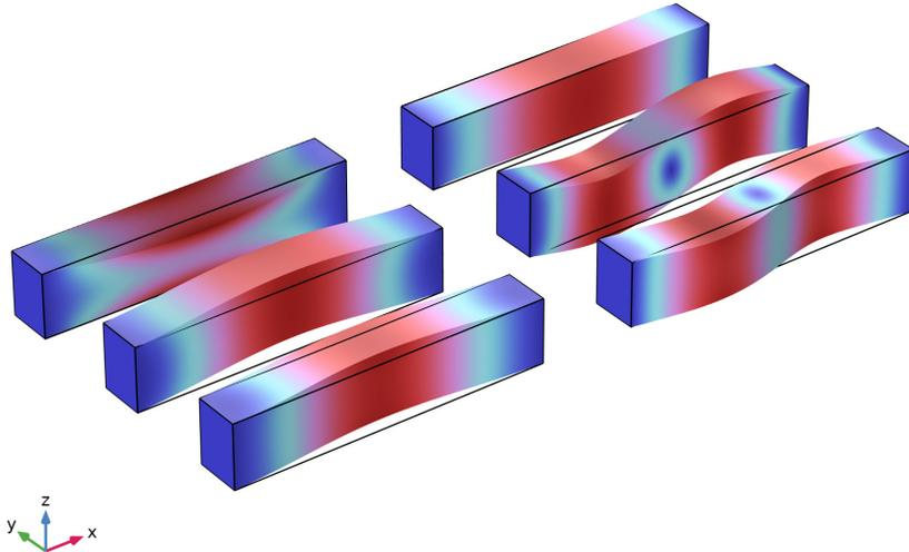
*Figure 2: The six constrained eigenmodes.*
