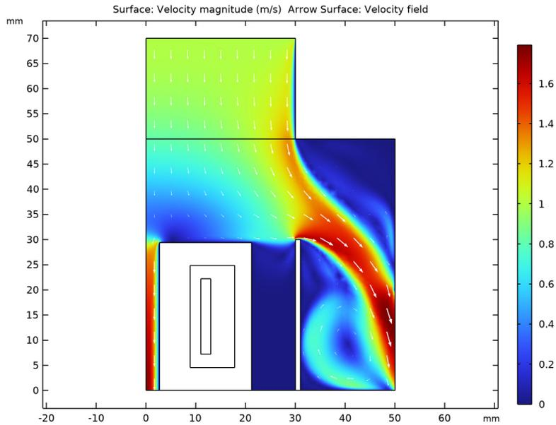
Figure 2: Magnitude and arrow plot of the velocity field.
