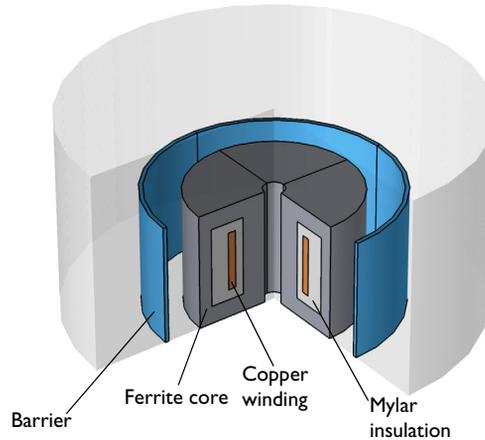
*Figure 1: 3D view of the model geometry.*
