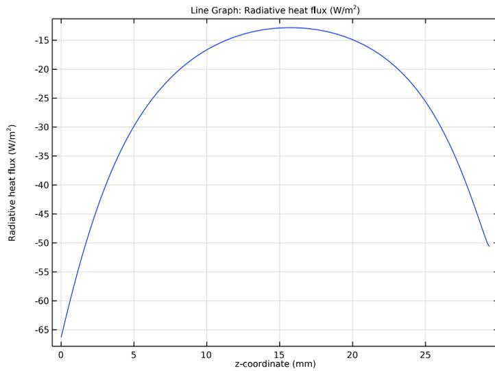
*Figure 4: Cross-sectional plot of the net radiative flux.*
