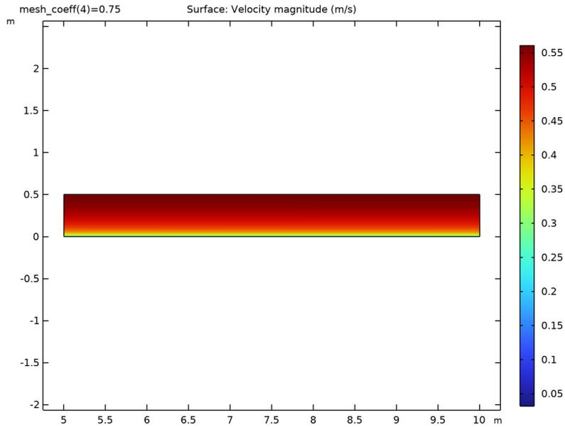
*Figure 1: Velocity field over the plate ( $x > 5$  m).*
