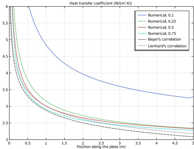
Figure 3: Comparison of the computed heat transfer coefficient with the heat transfer coefficient estimations based on Nusselt number correlations.
