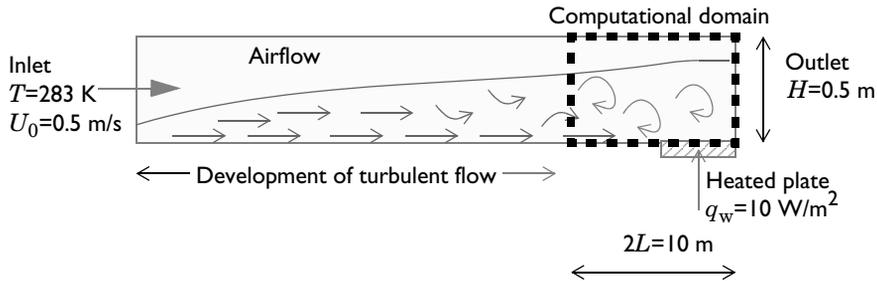
A plate of length  $L$  is heated with a constant heat flux  $q_w$  of  $10\text{ W/m}^2$  and placed in a turbulent airflow with average velocity  $U_0 = 0.5\text{ m/s}$  and temperature  $T_0 = 283\text{ K}$ . At the left boundary of the computational domain, the airflow turbulence is supposed to be fully develop. The airflow is heated over the plate.
