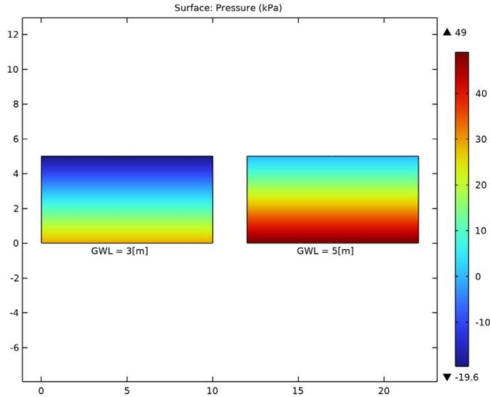
Figure 2: Pore pressure at different ground water levels.
