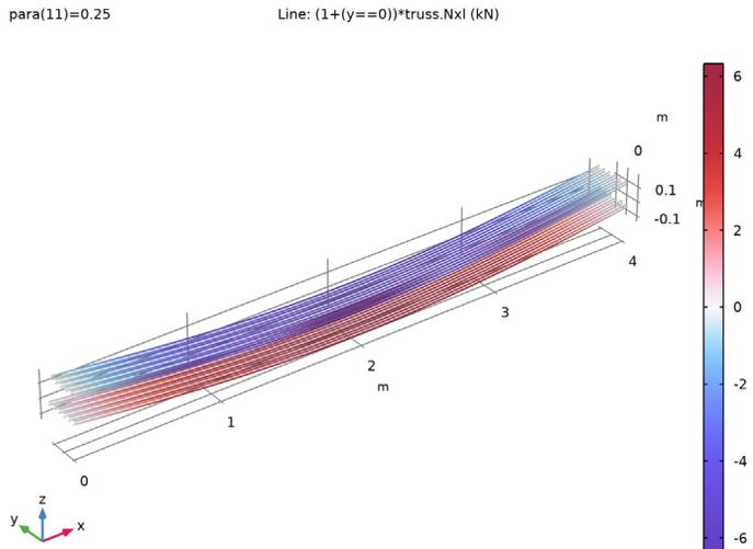
Figure 7: Axial force in the reinforcements bars. An extra multiplier is used on the bars in the symmetry plane in order to get the total force.
