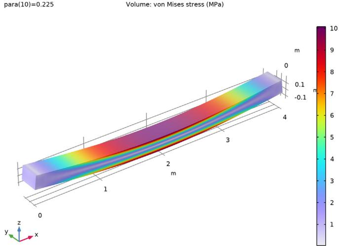
Figure 6: von Mises stress in a linear elastic beam after adding the fibers.
