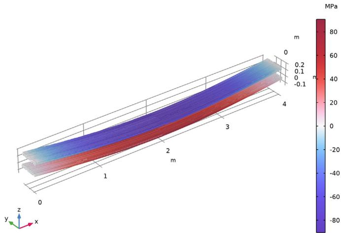
Figure 9: Axial stress in the steel fibers.
