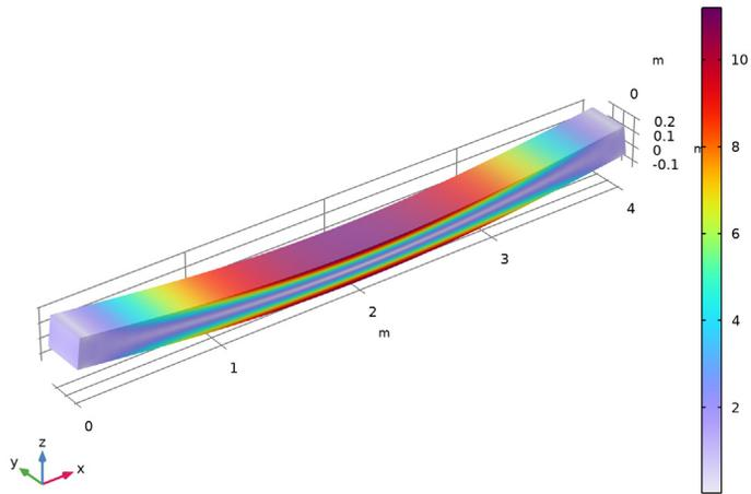
Figure 5: von Mises stress in a linear elastic beam after adding the reinforcement bars.
