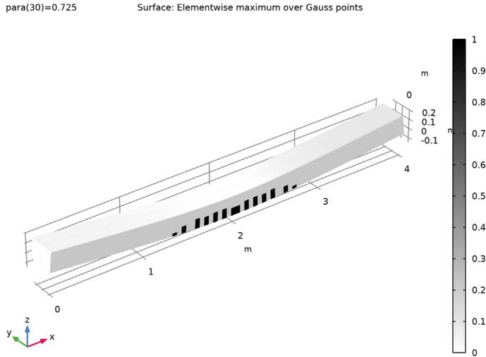
*Figure 14: Locations of cracks in Mazars damage model*
