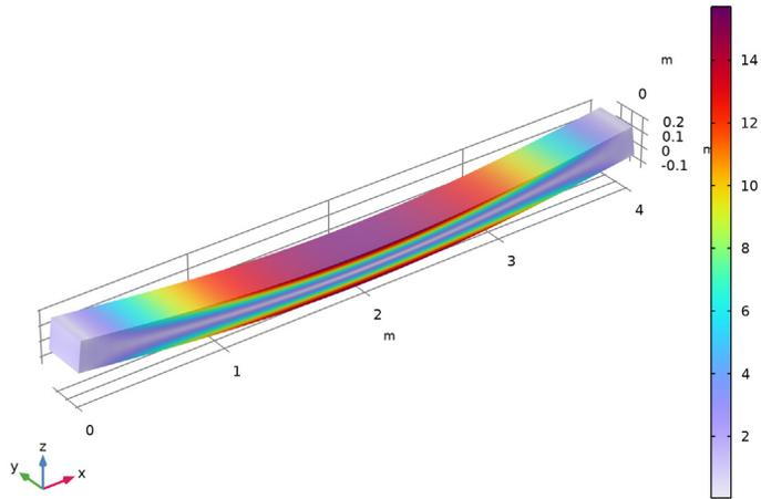
Figure 4: von Mises stress in a linear elastic beam.
