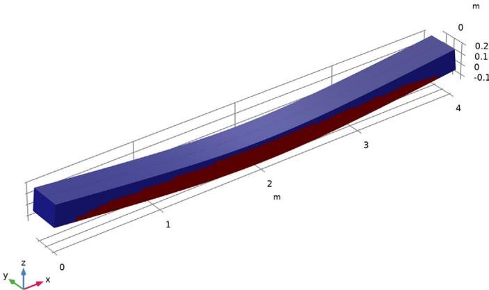
Figure 12: Plastic region in concrete with Ottosen model
