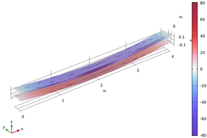
Figure 8: Axial stress in the steel rebars.
