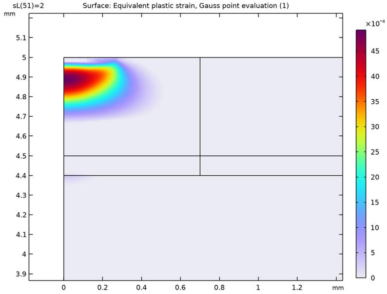
*Figure 5: Equivalent plastic strain after two load cycles.*
