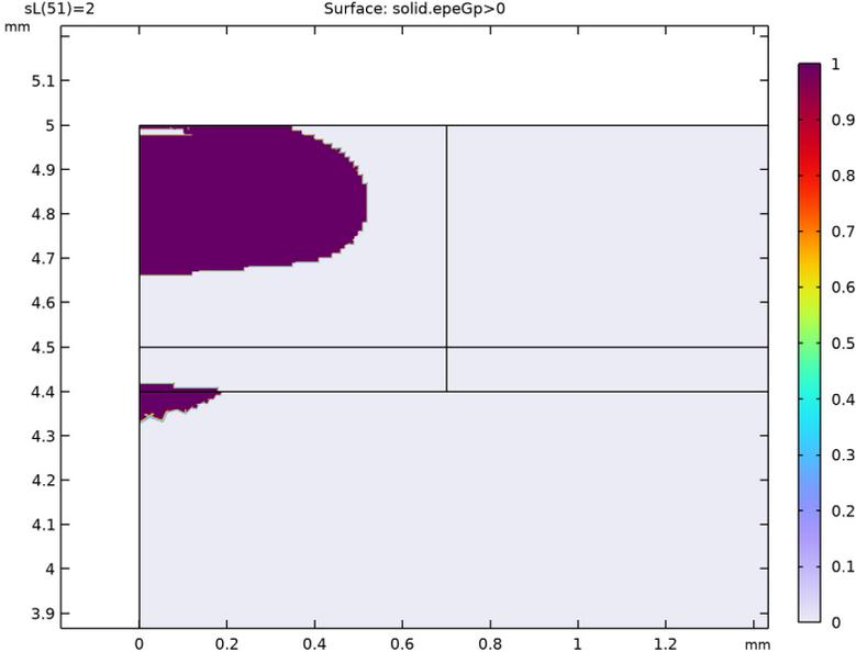
Figure 4: Plastically deformed volume after two load cycles.
