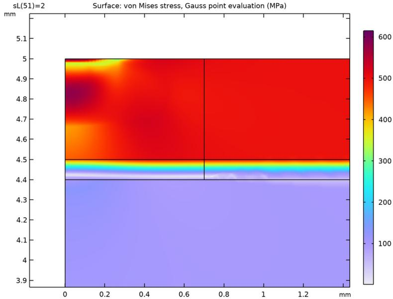
*Figure 3: The equivalent stress after two load cycles.*
