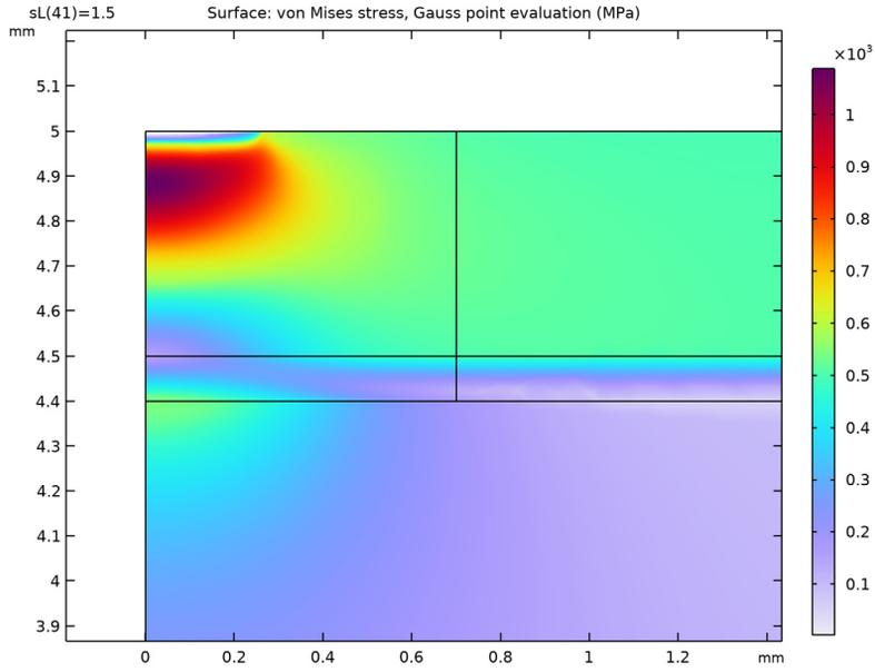
*Figure 7: Equivalent stress at peak load.*
