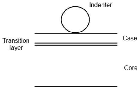
*Figure 1: Standing contact fatigue material testing.*
