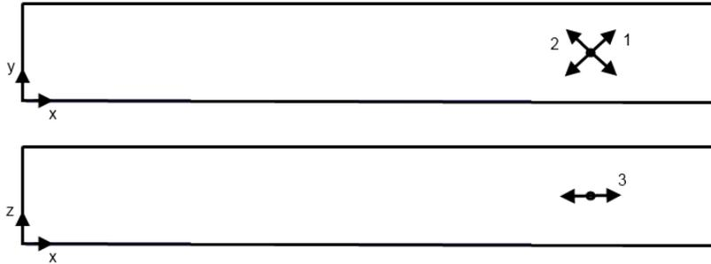
Figure 2: Location and orientation of the strain gauges.
