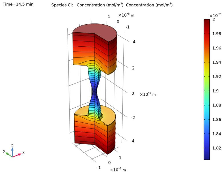
Figure 2: Chloride ion concentration (mol/m<sup>3</sup>) along with contour plot and electrode displacement in the cell after 14.5 minutes of operation.
