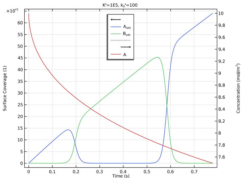
Figure 2: Surface coverages of species  $A_{\text{ads}}$  and  $B_{\text{ads}}$  and the concentration of A at the electrode surface for case 1) fast adsorption and fast charge transfer.
