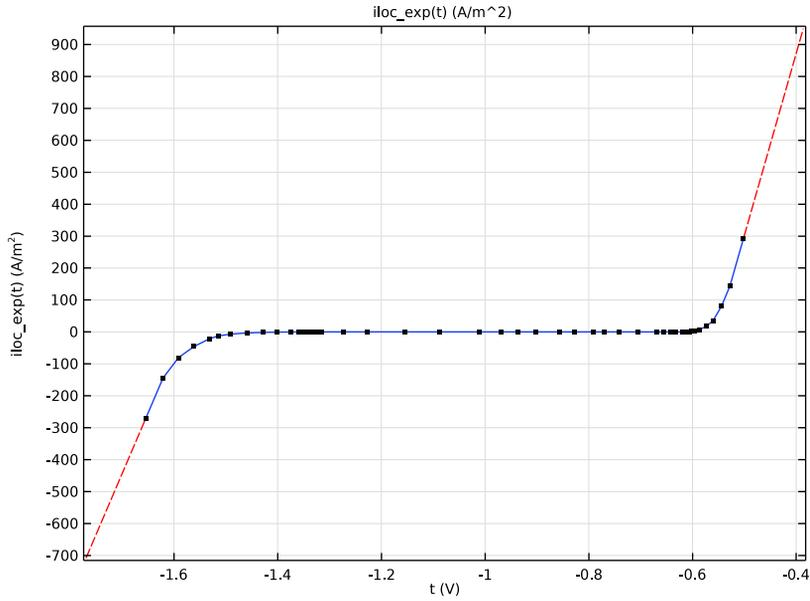
Figure 3: Polarization data for Al alloy.
