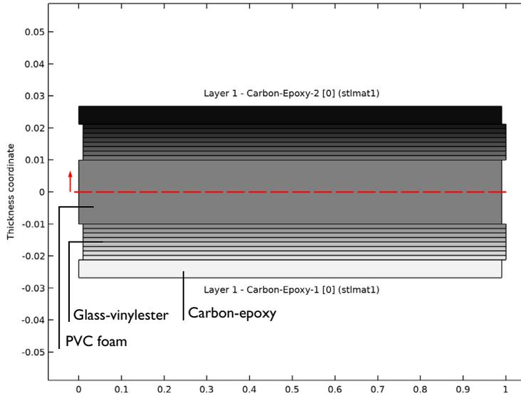
Figure 2: Through-thickness view of the laminate.
