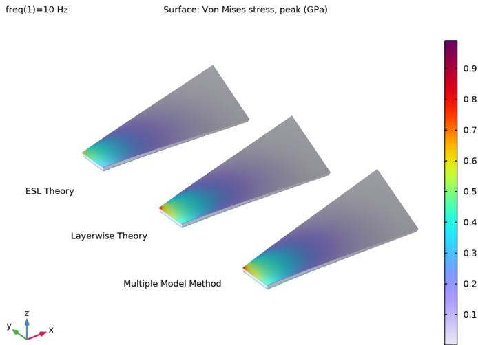
*Figure 6: Peak von Mises stress distribution in the composite blade.*
