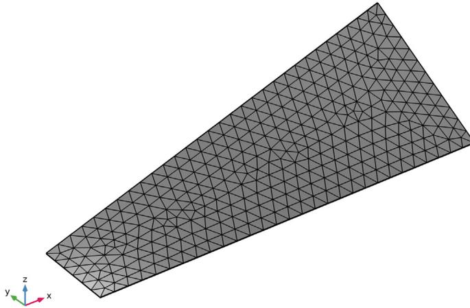
Figure 4: The mesh in the base selection.
