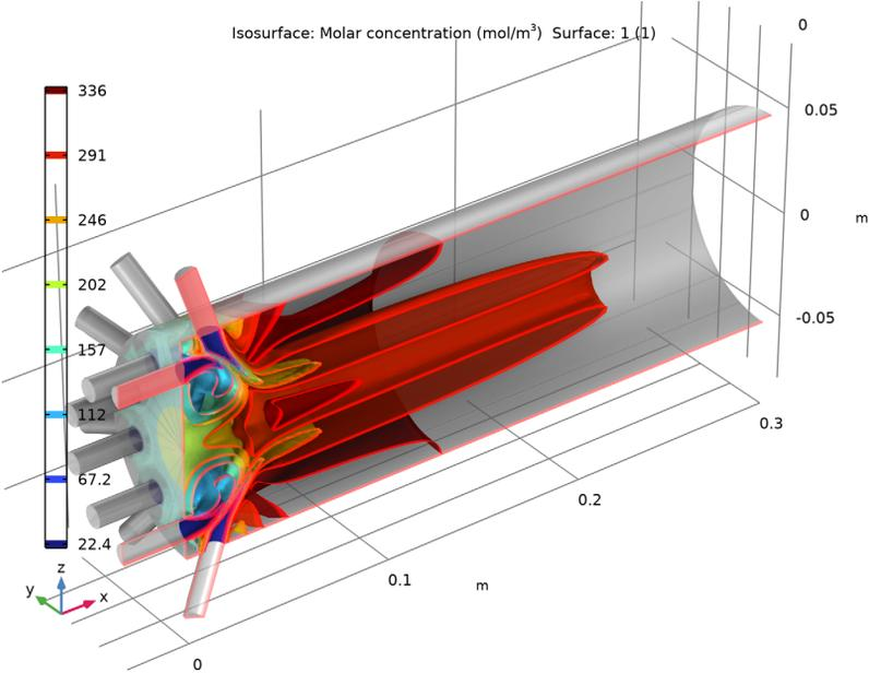
Figure 5: Isosurfaces for the concentration of L (mol/m<sup>3</sup>) visualized using a clip plane.
