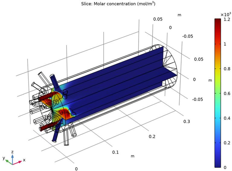
Figure 4: Concentration distribution of monomer A ( $\text{mol}/\text{m}^3$ ).
