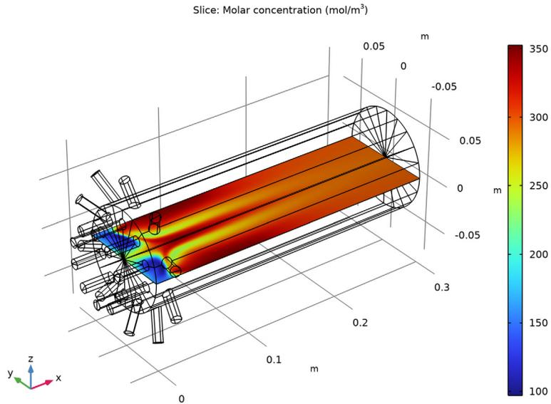
*Figure 6: Concentration distribution of polymer linkage,  $c_L$  (mol/m<sup>3</sup>).*
