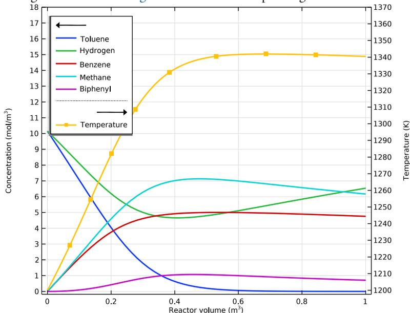
Figure 3: Concentration ( $\text{mol}/\text{m}^3$ ) and temperature (K) as function of reactor volume ( $\text{m}^3$ ) for a membrane reactor design with a continuous supply of hydrogen.
