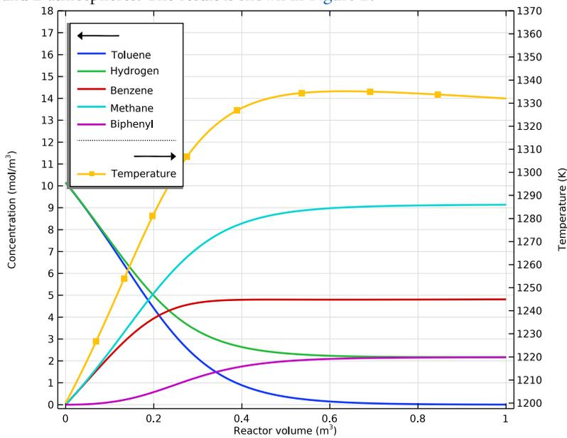
Figure 2: Concentration ( $\text{mol}/\text{m}^3$ ) and temperature (K) as function of reactor volume ( $\text{m}^3$ ) for a tubular reactor design.
