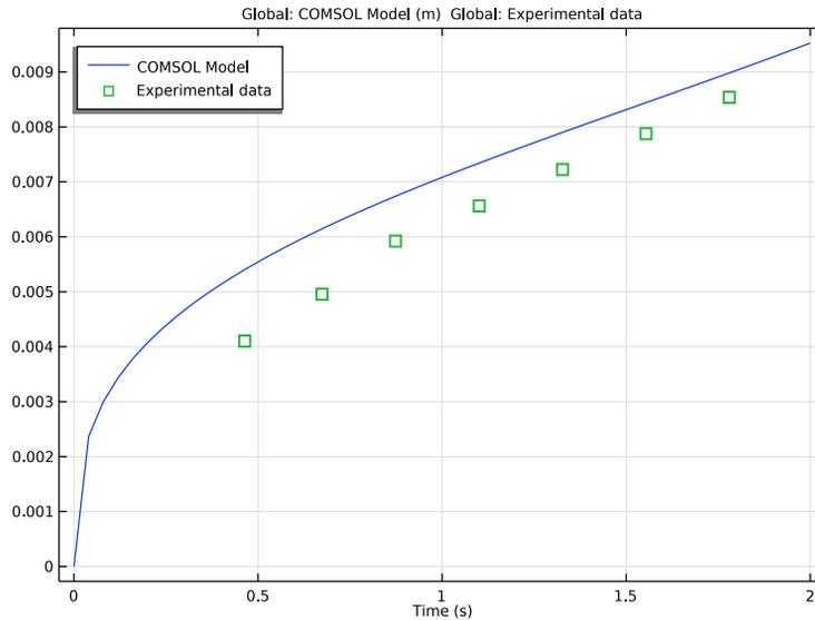
Figure 6: Displacement of the center of the catenary, relative to the anchors, as a function of time. The results are compared to experimental data from Ref. 2, which has an estimated error of approximately 15% (not shown in the plot).
