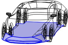
4 In the **Settings** window for **Boundary Layer Properties**, locate the **Layers** section.
