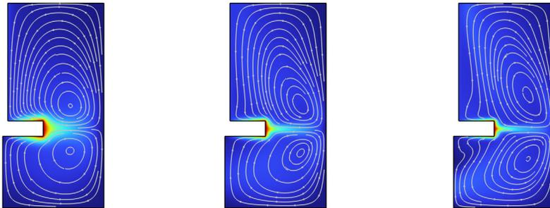
Figure 4: Results for angular velocities  $\omega = 0.5\pi$ ,  $2\pi$ , and  $4\pi$  rad/s. The surface plot shows the magnitude of the velocity and the white lines are streamlines of the velocity field.
