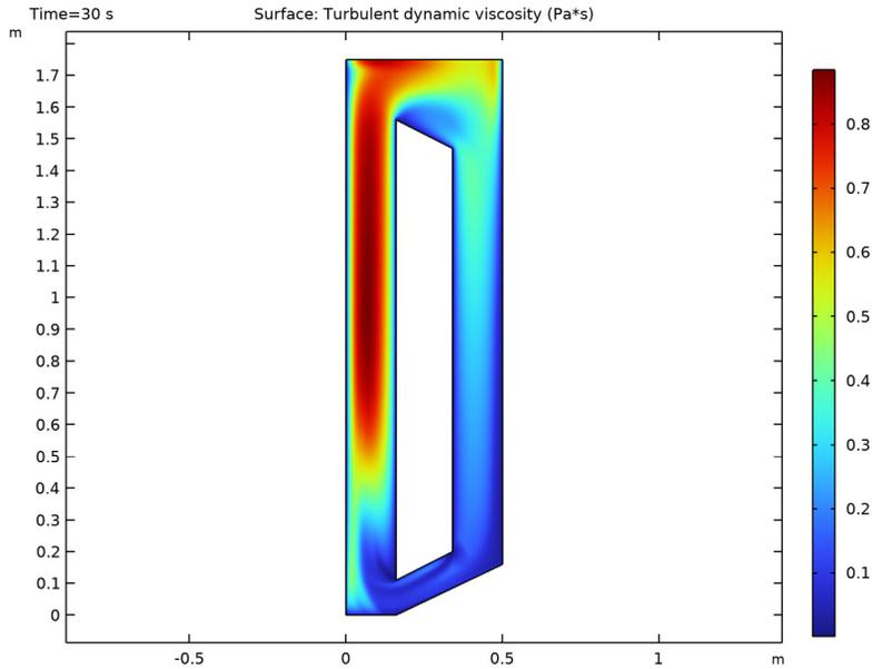
Figure 3: Turbulent viscosity in the symmetry plane.
