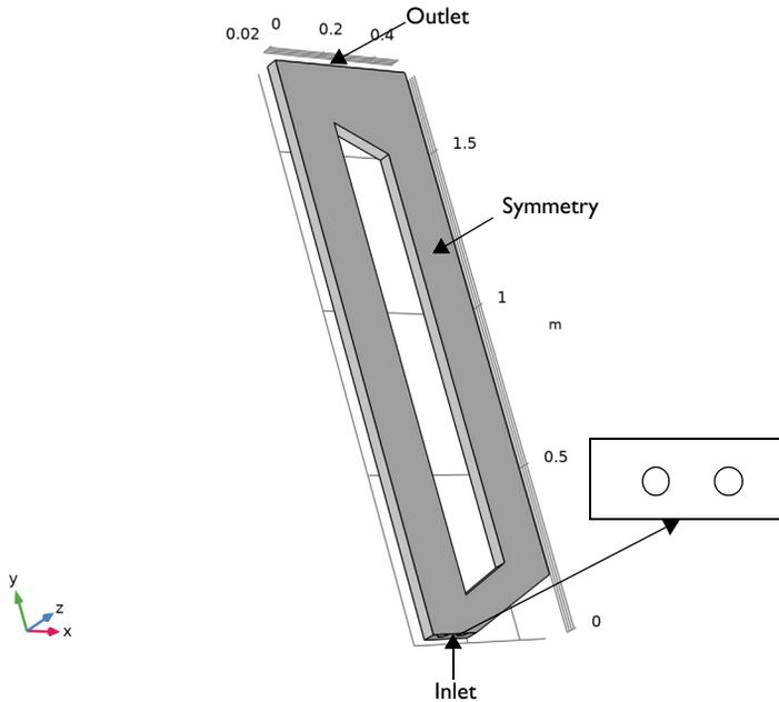
Figure 1: Model geometry for the airlift loop reactor.
