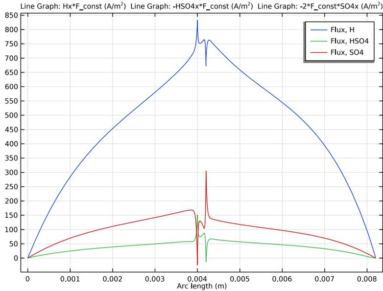
Figure 11: Sulfuric acid species fluxes along a horizontal line placed at  $y = h_{\text{cell}}/2$ .
