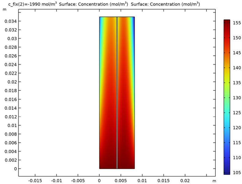
Figure 4: Concentration of the  $V^{2+}$  (left compartment) and the  $VO_2^+$  (right compartment) ions for a membrane charge concentration of  $-1900 \text{ mol/m}^3$ .
