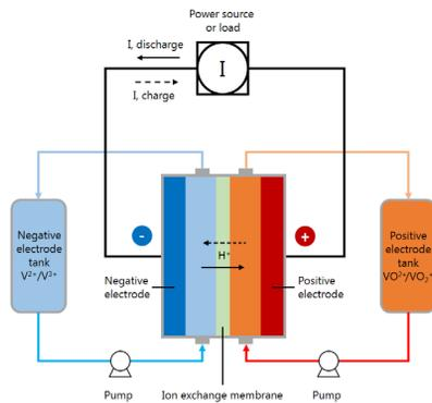
*Figure 1: Schematic of a vanadium redox flow battery system.*
