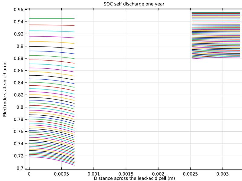
Figure 12: State-of-charge during the one-year self-discharge simulation.
