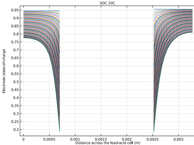
*Figure 10: State-of-charge decrease during the 20C discharge simulation.*
