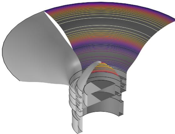
*Figure 3: The optimization results (top) are shown together with the initial design (bottom).*
