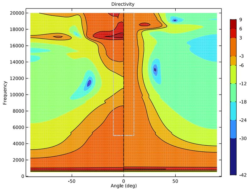
Figure 5: Directivity plot of the initial design (left) and optimized design (right). The colors show the deviation from the target sound pressure level. Black lines mark the  $\pm 3$  dB and  $\pm 6$  dB limits. The gray box marks the frequencies and locations used during the optimization.
