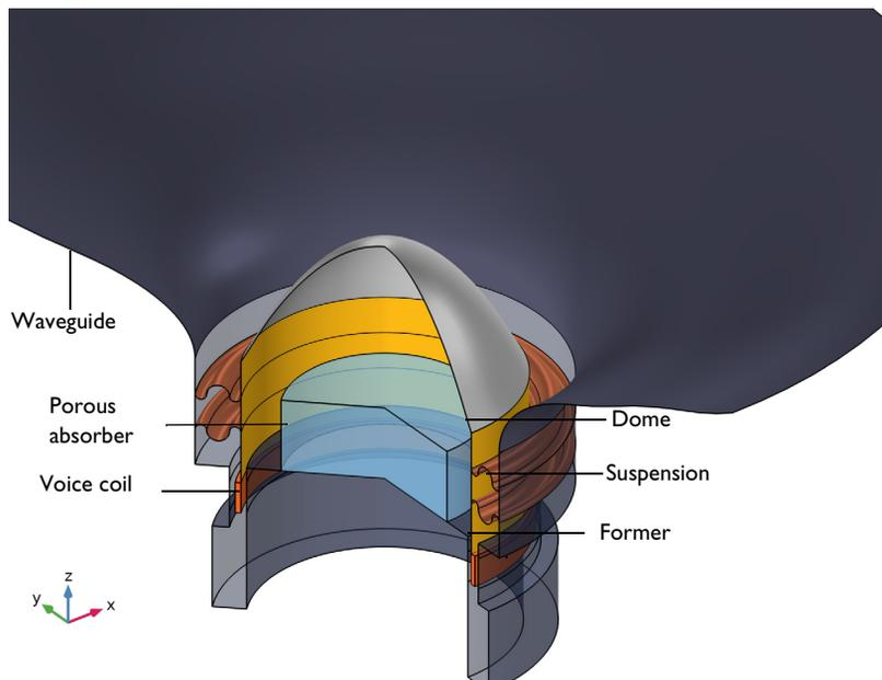
*Figure 1: Geometry of the initial tweeter design.*
