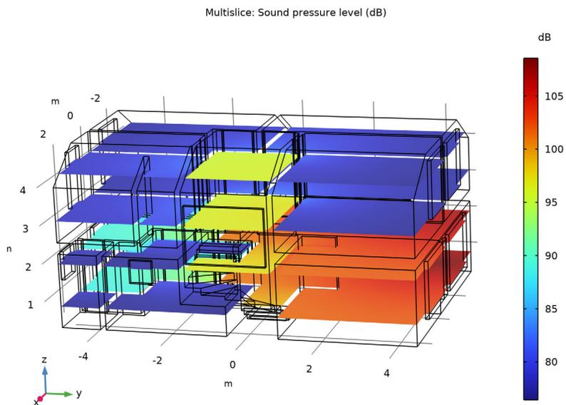
*Figure 2: SPL on horizontal slices of the model.*
