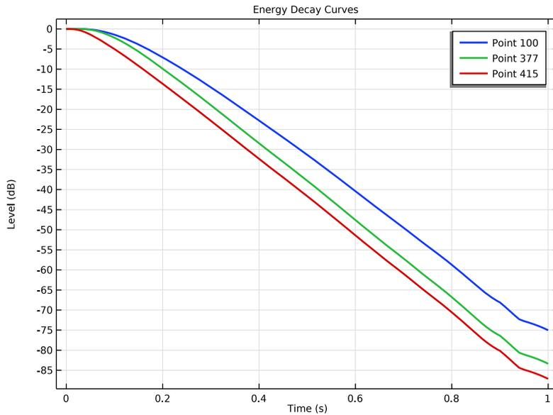
Figure 8: Energy decay curves from three different rooms.
