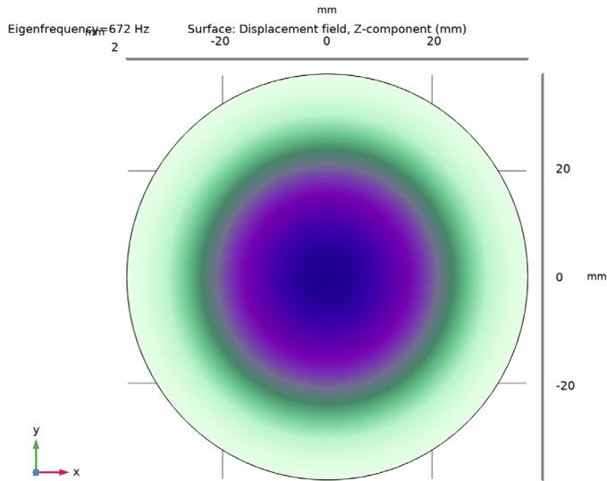
*Figure 1: First structural mode displayed by vertical displacement.*
