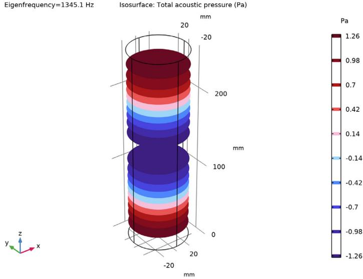
Figure 4: Second acoustic mode displayed by pressure isosurfaces.
