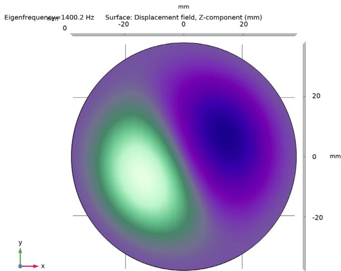
Figure 2: Second structural mode displayed by vertical displacement.
