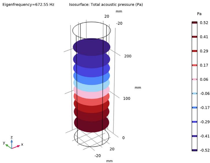
Figure 3: First acoustic mode displayed by pressure isosurfaces.
