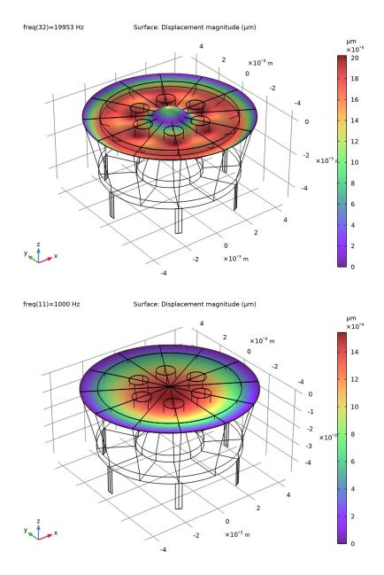
Figure 5: Diaphragm deformation at f = 20 kHz (top) and f = 1 kHz (bottom).
