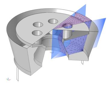
Figure 3: Geometry of the BK 4134 microphone. The computational mesh is reduced to 1/12 of the geometry using symmetries.
