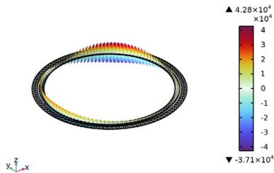
The longitudinal current density moves back and forth within the cross section with an average hovering around zero, as discussed before.
