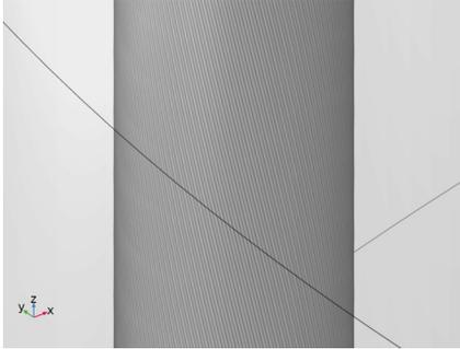
At first the cable looks stretched, because the camera is using the latest parameter values while the geometry has not yet been rebuilt.
