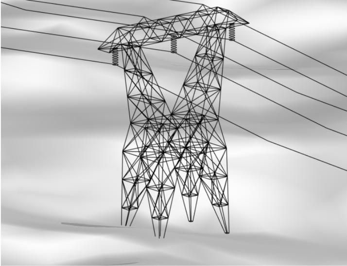
*Figure 1: The geometry of the transmission tower. The two shielding lines can be seen on top, while the three phase lines are held by the insulators.*
