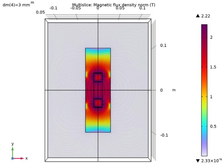
Figure 7: Magnetic flux density and magnetic flux streamlines in a slice parallel to the plate upper surface for the initial distance of 3 mm between the plate and magnet.
