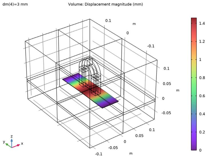
Figure 5: Displacement of the plate for the initial distance of 3 mm to the magnet.
