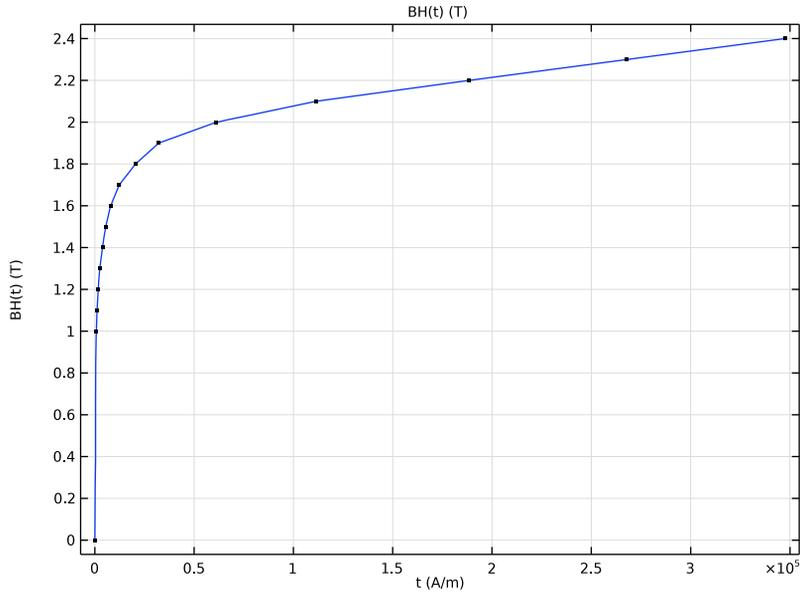
Figure 3: BH curve for soft iron.
