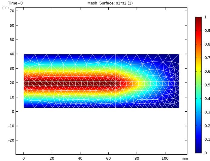
*Figure 2: Parameterization of the deformed domain. The parameterization is used to rigidly move the plate and deform continuously the mesh in the surrounding air domain.*
