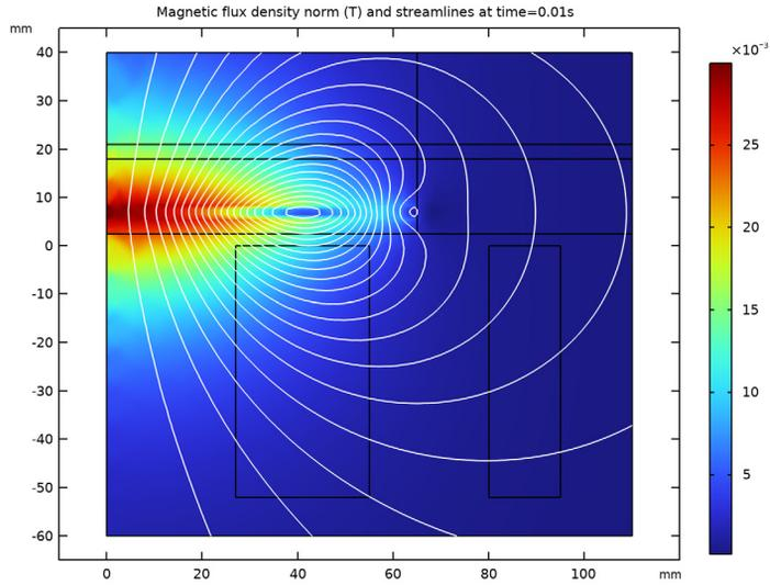
Figure 4: Magnetic flux density norm and field lines at  $t = 0.01$  s.
