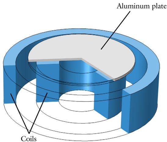
The application models the dynamics of the plate in the time domain, from when the coils are energized to the end of the transient after 1.7 s. The results, and, in particular, the position of the plate, are compared with the experimental data available from the TEAM problem specification.
