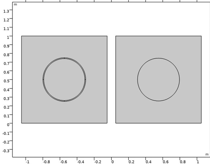
The geometry on the left side describes the full fidelity model. The geometry on the right side replaces the thin layer with a boundary in order to use the **Contact Impedance** feature.
