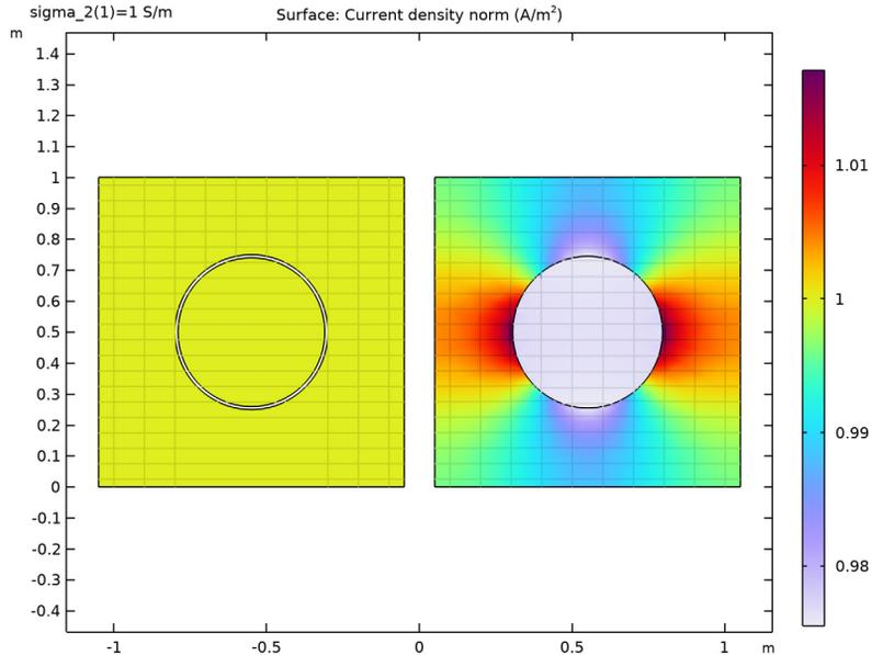
*Figure 3: A surface plot of the current density norm, together with isolines of the electric potential and streamlines indicating the current direction. The contact impedance boundary condition (right) prevents any tangential current flow.*
