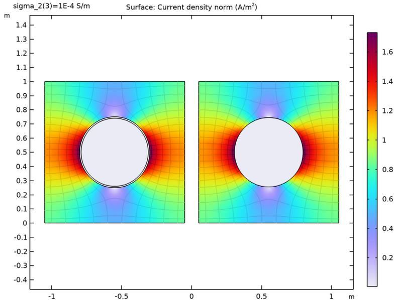
*Figure 2: A surface plot of the current density norm, together with isolines of the electric potential and streamlines indicating the current direction, for the case of a thin layer of material that has a high impedance. The full fidelity and contact impedance solutions are almost identical.*
